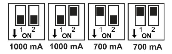
The driver will be shipped out of factory with both switches set to ON (700mA).
